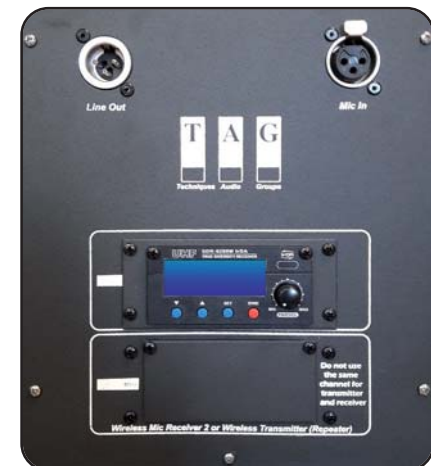
2 slots for: UHF Receiver or/and UHF Transmitter
