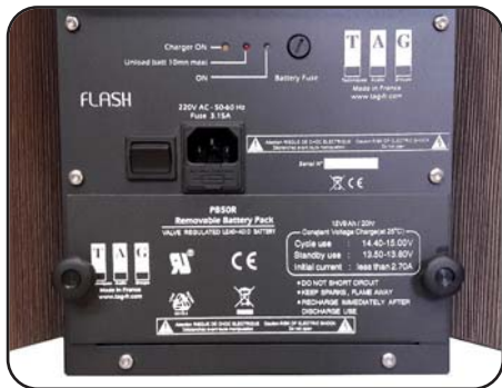
AC main and/or Battery 7 Ah - 12V (6 - 9 h)
