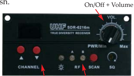
Selection of the channel LED A et B
