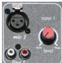
Input N°1 is equipped with 1 XLR (3 pins) mic input, 1 line input equipped with 2 RCA connectors and a volume control. The input selection is automatic. If both inputs are connected, you can use them simultaneously
