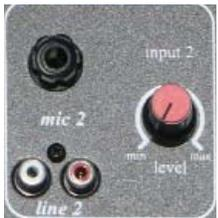
Input N°2 is equipped with 1 stereo Jack (6.35mm) mic input, 1 line input equipped with 2 RCA connectors and a volume control. The input selection is automatic. If both inputs are connected, you can use them simultaneously.
